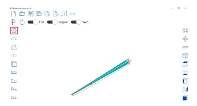
3. The below window will appear after clicking on the setting tab. The regions can be added and subtracted based on the requirements by using the highlighted tab. The Blade name and the name of the regions are also editable.
