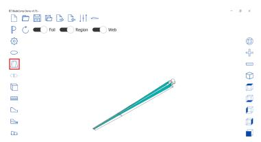
9. As per the data for the geometric shape, the region splits on index 30, so splitting 30, 30 for each region, and click Ok.
