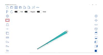
5. Select the four profiles and add the relevant information which fulfils the requirements of the geometric shape of the 13-meter-long blade. Add the required data in the table on the right side of the window (in the form of X and Y) for each profile, and click Ok.
