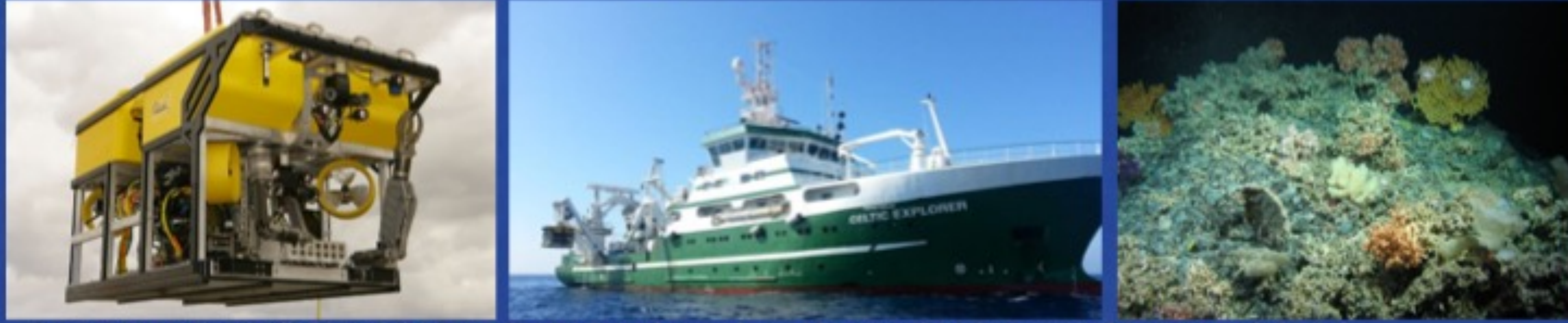
Fig. 1: ROV Holland 1 (left) and the RV Celtic Explorer (centre) used for sampling deep sea cold water reefs (right).
