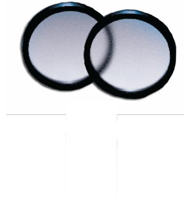
(b) Photograph of the holographic diffuser used in the setup
