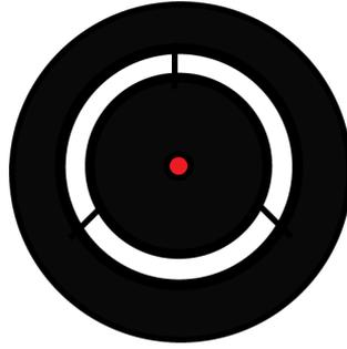
Figure 7.2: Example of the proposed redesign of the illumination targets for the subjective techniques. The simple addition of a filtered hole highlighting the desired point of fixation.
